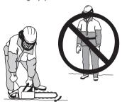
Always hold the saw with both hands. The right hand should be on the rear handle, and the left hand on the front handle. All people, whether right or left handed, should use this grip. Use a firm grip with thumbs and fingers encircling the chain saw handles.
